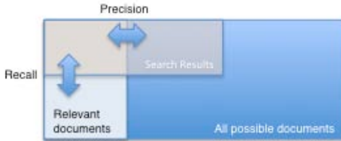
Figure 2.3 An illustration of precision and recall in the context of search results
